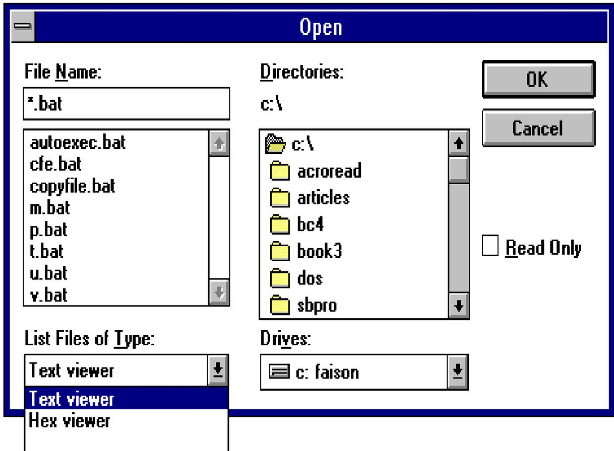
Figure 4 - The viewer selection combo box in the File Open dialog box used by OWL.
